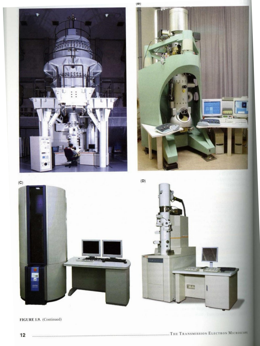
FIGURE 1.9. A selection of different commercial TEMs: (A) JEM 1.25 MeV HVEM. Note the size of the instrument; often the high-voltage tank is in another room above the column. (B) Zeiss HRTEM with a C, corrector and an in-column energy filter. Note the large frame to provide high mechanical stability for the highest-resolution performance. (C) Hitachi 200 keV dedicated STEM; note the absence of a viewing chamber. Such instruments are often designed to aid failure analysis for the semiconductor device manufacturers. Specimens thinned from wafers on the production line can be easily transferred and examined. (D) JEOL 200 keV TEM/STEM; note also the absence of a viewing chamber. (E) Nion 200 keV ultrahigh vacuum SuperSTEM; the only US-manufactured (S)TEM and current holder of the world record image resolution (F) FEI Titan. Comparison with Ruska's instrument (Figure 1.1), which is 70–80 years older than these instruments, is instructive.
